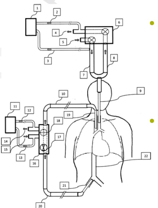
30 minutes indirect calorimeter connected to the ventilator
